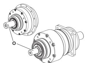
① Only the "self-contained version" gearbox variant with a drive shaft [O] is not intended for motor mounting. It is possible to drive the gearbox directly via the drive shaft, e.g. by means of a belt pulley.
