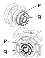
The slip-on shaft / hollow shaft / hollow shaft interface [Q] is axially secured to the load shaft by means of a shrink disk connection. If a gearbox with shrink disk [P] was ordered, then it is already mounted.
