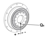
To ensure reliable lubrication and sealing of the gearbox, observe the minimum swivel angle at the output.
