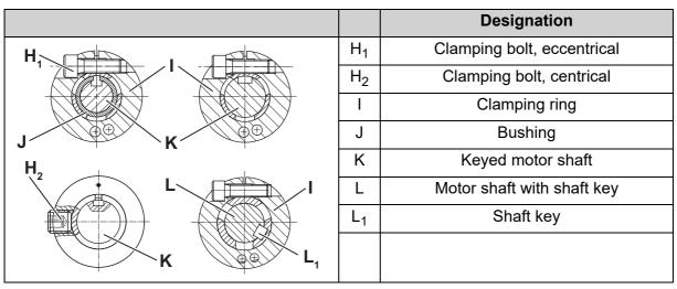
Tbl-6: Arrangement of motor shaft, clamping bolt and bushing
